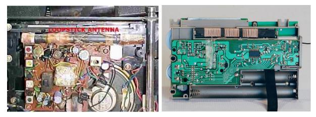
How they work is that any loop of wire has a magnetic field. When that magnetic field picks up the magnetic field energy lines from the transmitter signal, some of that energy is converted into electricity and fed into the radio amplifier circuits.
